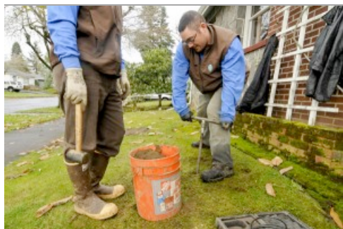
Conor McGeehan, left, and Toshio Sagara, field supervisors with Soil Solutions, take soil samples from the yard of a Southeast Portland home to check for contamination from an underground heating oil tank. (Photo by Sam Tenney/DJC)
