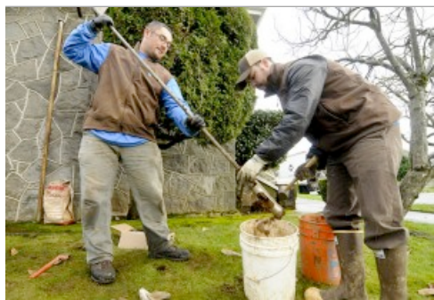
Toshio Sagara, left, holds an auger as fellow Soil Solutions field supervisor Conor McGeehan removed dirt from the bit while taking soil samples. (Photo by Sam Tenney/DJC)
